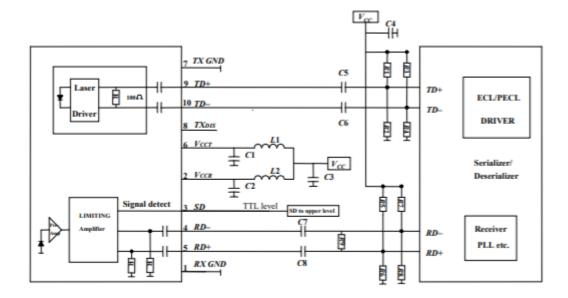
C1/C2/C4/C5/C6/C7/C8 = 100 nF  $C3 = 4.7 \mu\text{F}$   $L1/L2 = 1 \mu\text{H}$  R1/R2/R3/R4/R5/R6/R7/R8/R9 Depend on SerDes
